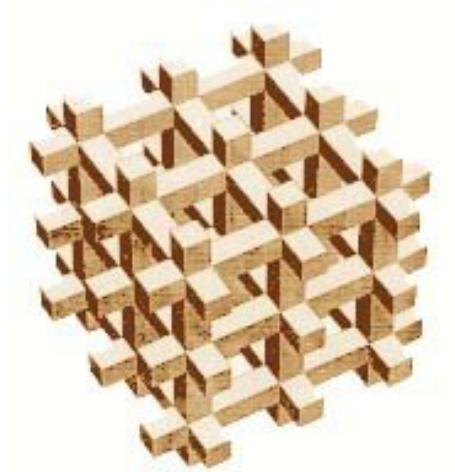
Figure 1: Intersecting Square-Rod 構造 ( 3 \times 3 \times 3 )
